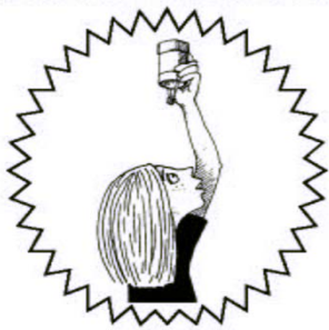
Correct Way To Hold A Homemade Densiometer
