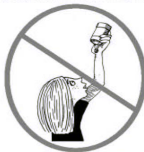
Incorrect Way To Hold A Homemade Densiometer
